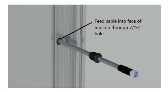
STEP 6: Push grommet into hole until grommet shoulder is firmly against face of mullion
