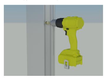
STEP 2: Deburr Drilled Hole
