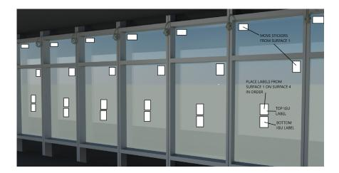
**NOTE:** Prior to installing frames on building (either in-shop or on-site) move stickers from side 1 to side 4 in the order they are in the frame from top to bottom
