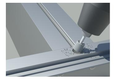
Drill and De-burr 7/16" Diameter hole in the face of the mullion where cable is to be installed. See approved integration and shop drawings for locations. Note: If holes are CNC cut and clean, deburring may not be necessary.
