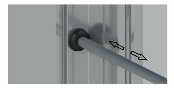
STEP 8: Clean away excess caulking that has squeezed out of the hole
