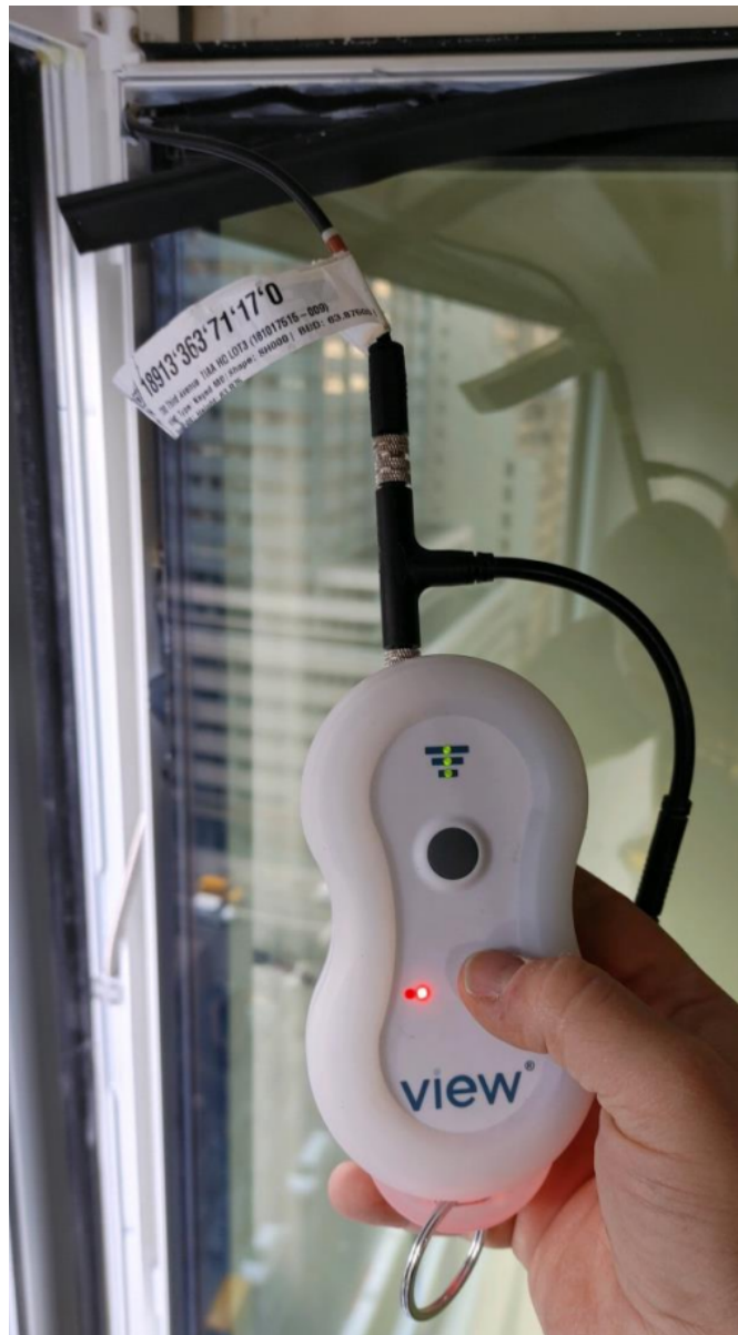
Fig. 5: Plugging the SWC into GTT
