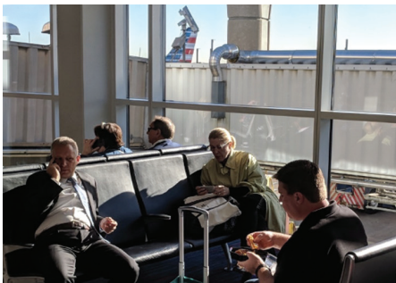
Observations of discomfort with lighting conditions at Gate A25 - Low-E glass. On the left, a passenger shielding a device from glare, and on the right, a passenger wearing sunglasses while facing the windows
